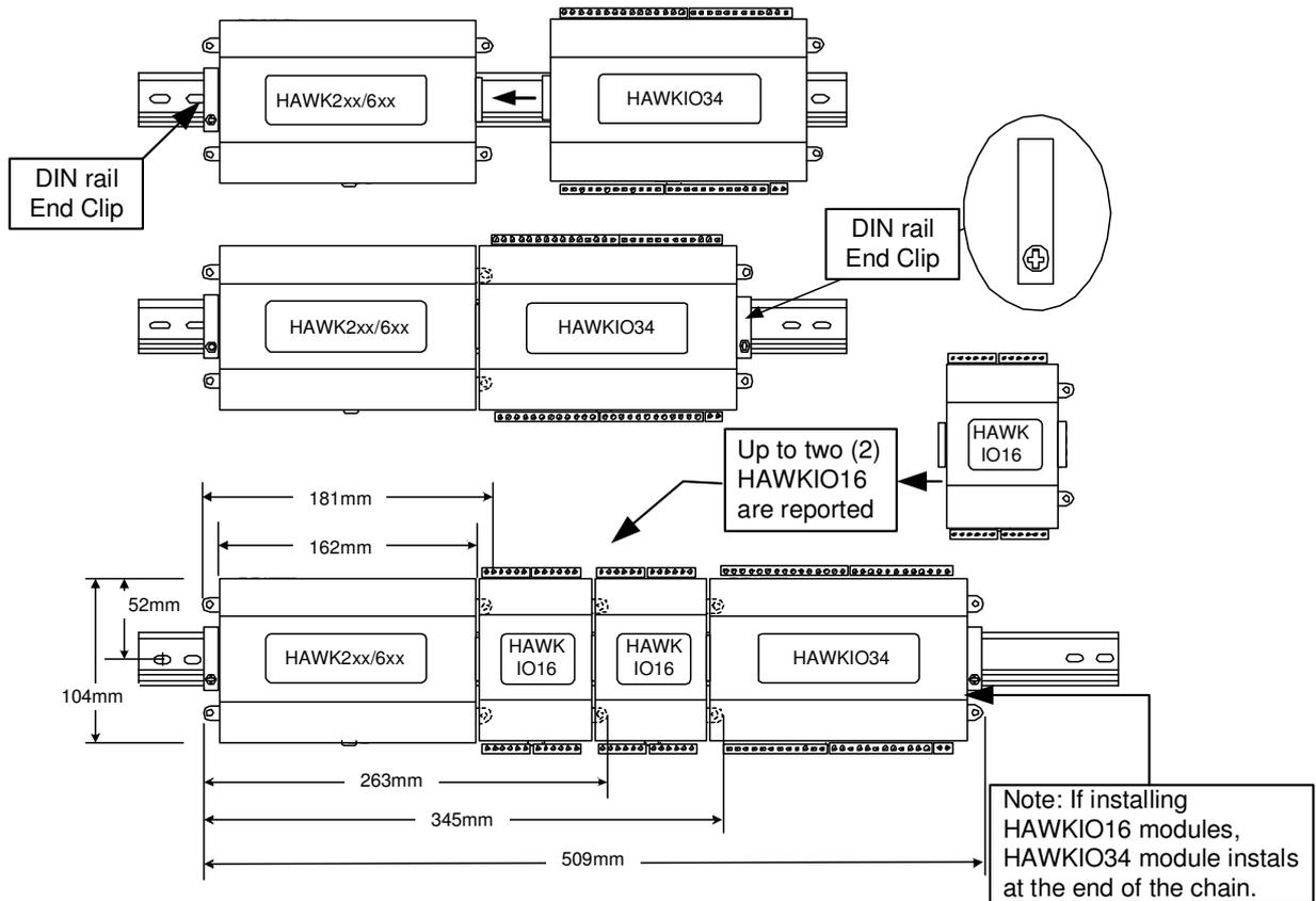
**Fig. 1. HAWKIO34 module mounting details**
