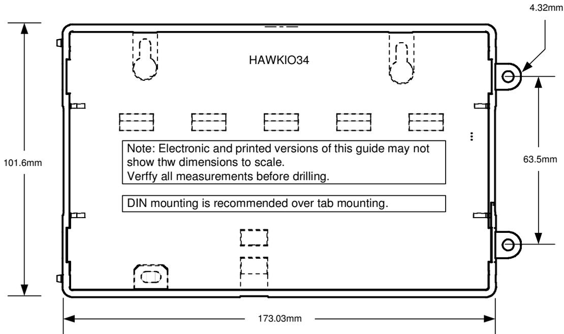
Tip: When mounting HAWK, you can simplify any future removal or replacement of it by not installing screws in its "accessory module side" tabs (see below)
