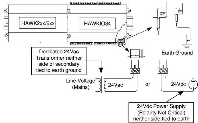
**Fig. 3. CLAXHAWKIO34 earth ground connection**
