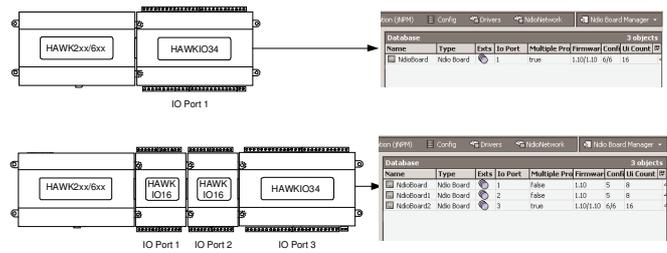
**Fig. 10. NdioBoard assignment is determined by proximity order to HAWK**
